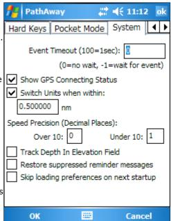
**Track Depth in Elevation Field**: For nautical GPS devices with Depth reporting, PathAway can be set to record these depths to the track log instead of elevation.
