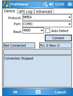
Note: The most common baud rate for most GPS devices is 4800 BPS. Next is 9600, followed by 57,600.
